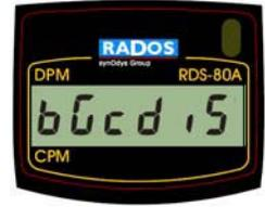
*Note: The background correction will be only performed when the DPM unit is activated. In other words, when the CPM unit is active, no background correction is carried out even if the bGc on was selected.*
