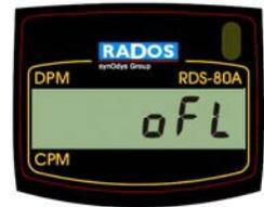
The overflow alarm cannot be reset.
