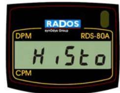
Press the push button shortly to return to the main menu or wait 7 seconds to return to the dose rate display.
