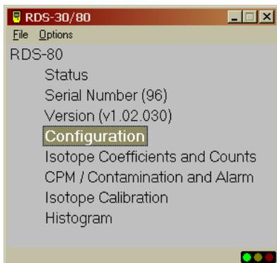
The Configuration Software (CSW) is used to check the status of the instrument, to change its operational parameters and to set-up the histogram operation (for details see the CSW Configuration Software for RDS-80A User's Manual)
