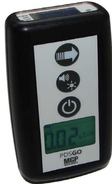
The PDS-GO is a lightweight, small, sensitive, personal gamma radiation detector, designed to meet the ANSI N42.32 radiation detection requirements. It has been designed using the latest state-of-the-art electronic components including the advanced technology of Silicon photomultiplier as a detector.
