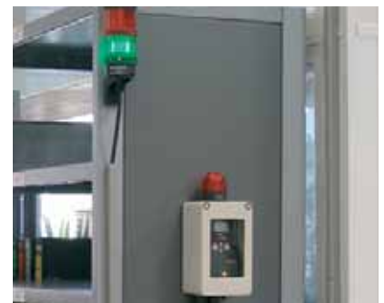
RadEye Area Monitor for neutron radiation
